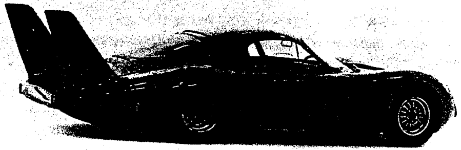
Fig. 7-2. The 1966 Peugeot CD, Le-Mans racer, which used vertical fins to increase lateral stability (courtesy of Peugeot Motors of America).
